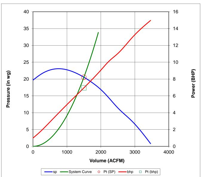
This configuration is compliant with CEC regulations (suitable for use in California). FEI: 1.38
