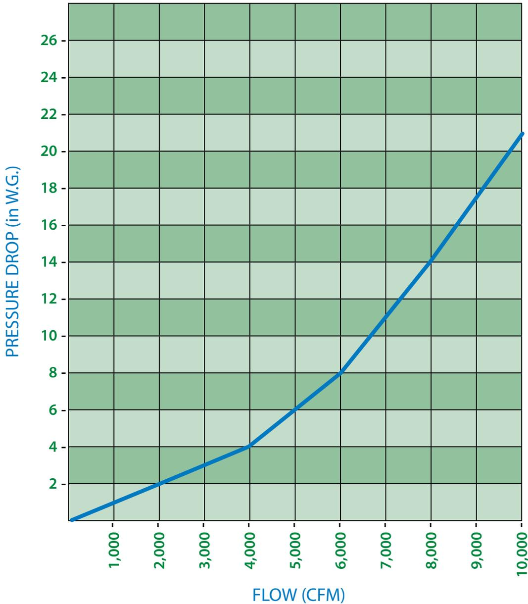
**Note:** Pressure drop readings were recorded using 4MM pellet carbon media in vessel.
