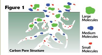
The removal of  $H_2S$  requires a thin water layer in the carbon pore structure to promote the reaction between  $H_2S$  and the carbon surface (see below). DARCO  $H_2S$  is very hydrophilic, allowing it to work well in environments with a wide range of relative humidity. DARCO  $H_2S$  has been proven effective in gas streams with relative humidity from 30% to 100% (saturated).
